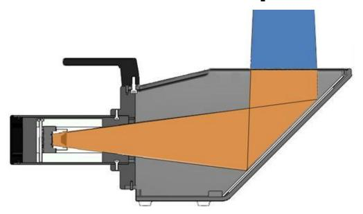
This diagram shows how the radiation beam is converted to visible light by the 20 x 20 cm scintillator and then reflected off the 45 degree mirror to the USB digital camera. The PC then captures beam images and performs measurements.
