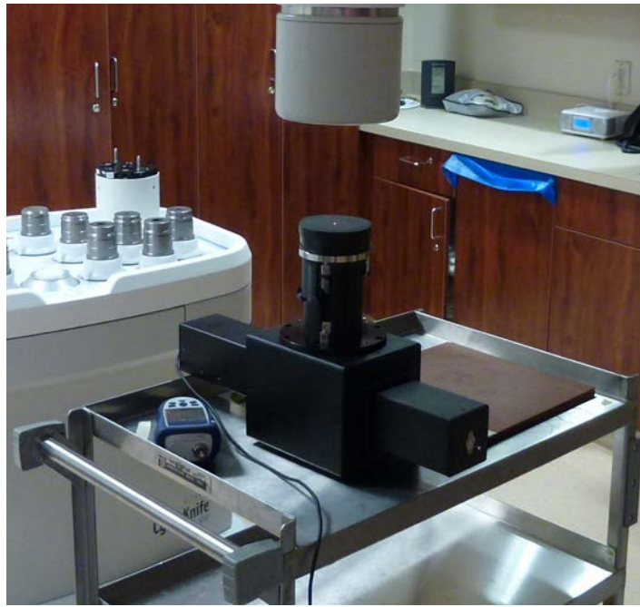
Figure 5 – IBAC detached from the Iris with the scintillator at 57.7 cm SAD
