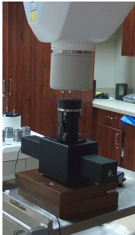
Figure 6 – IBAC supported by two 5 cm spacers with the scintillator at 47.7 cm SAD
