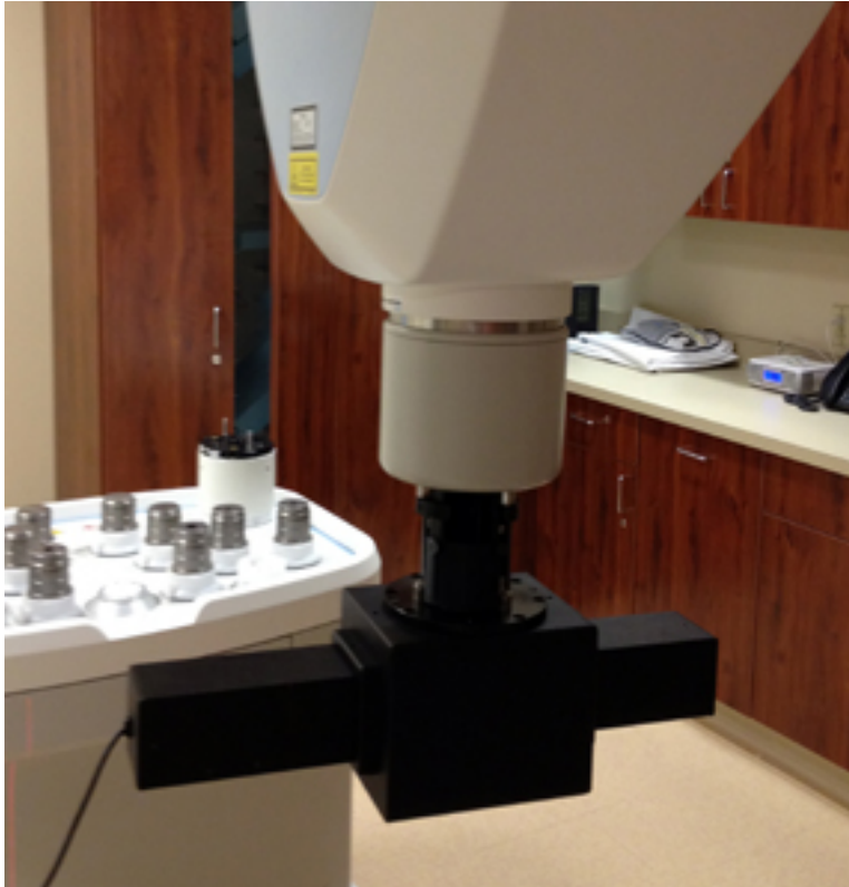
Figure 2 – The IBAC is shown attached to the CyberKnife Iris with the scintillator module access door open.
